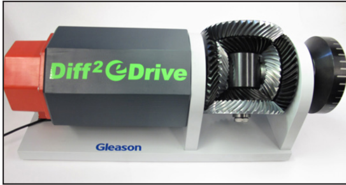
Figure 10 Prototype transmission with motor—Ratio 81.
