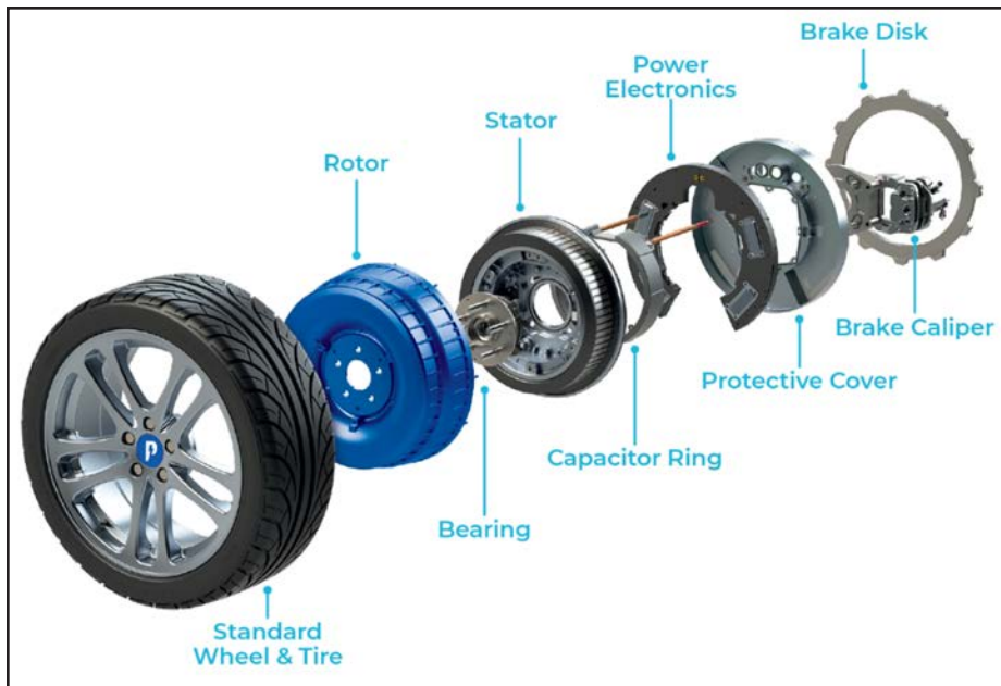
Figure 10 In-wheel direct drive motor (Ref. 10).
