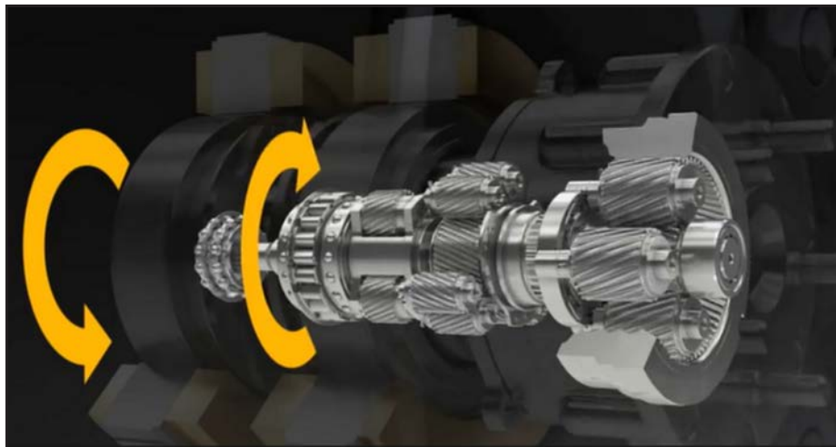
Figure 11 Double-wheel hub motor with transmission (Ref. 11).
