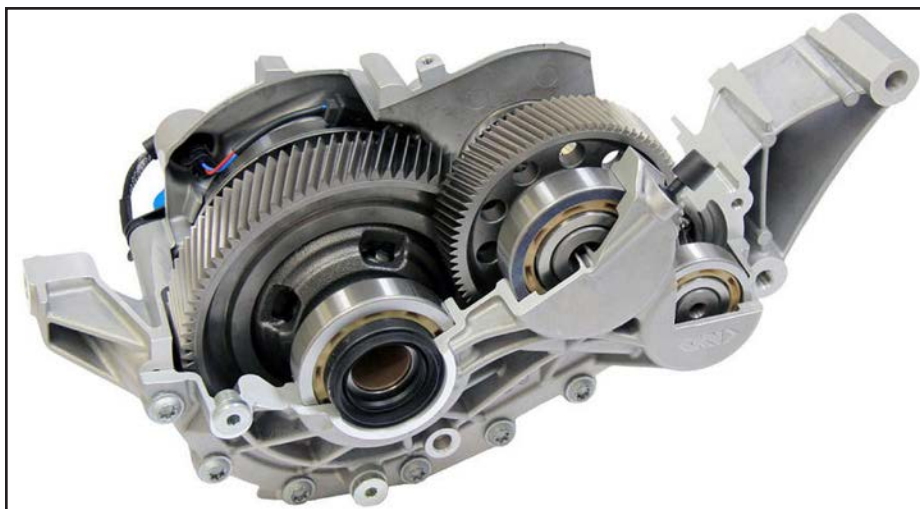
Figure 4 Two-stage and single-speed electric vehicle transmission — ratio 12.5 (Ref. 3).
