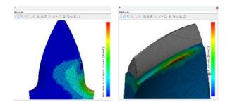
A 2D FEM calculation is sufficient to determine the tooth root stress caused by grinding notches. A 3D FEM calculation is recommended if the influence of a flank modification is to be taken into account.
