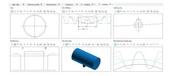
Sizing of the hob is available with consideration of shaft interference, shortest processing time and others. Additional sizing functionalities are implemented such as calculation of smallest hob width, maximum chip thickness and feed mark depth.
