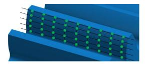
GAMA formats can be used for quick and secure data transfer between KISSsoft and a Gleason metrology system. GAMA enables the transfer of macro geometry data of cylindrical gears directly to the metrology system. The export format for GDE is defined in the VDI/VDE 2610 guideline. This guideline provides an exact and unique method for describing gear geometry and manufacturing data.
