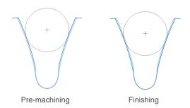
A flattened measuring ball can be defined for spline profiles, to prevent the tooth root from being touched.
