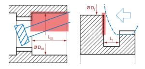
For outer gears the collision check is done between the tool front side and the shaft contour. For internal gears, the collision check is done between the tool shank and the shaft bore diameter. For a detailed analysis, the verification for a potential collision by Gleason is recommended.
