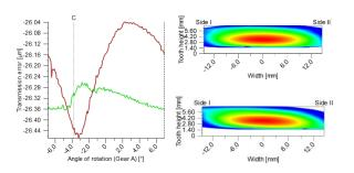
The loaded tooth contact analysis shows the behavior under load, such as stress distribution and contact pattern. The transmission error (PPTE) is used to analyze the noise excitation of gears.
