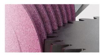
Both grinding processes – profile and threaded wheel grinding – are simulated in KISSsoft and the resulting root rounding is graphically displayed.
