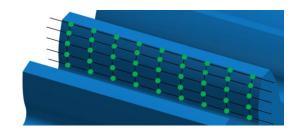
GAMA formats can be used for quick and secure data transfer between KISSsoft and a Gleason metrology system. GAMA enables the transfer of macro geometry data of cylindrical gears directly to the metrology system.
