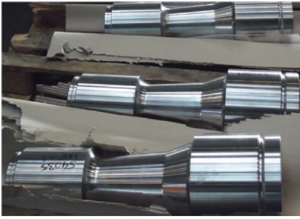
Figure 8—Flexpin pins, awaiting transport to heat treatment.
