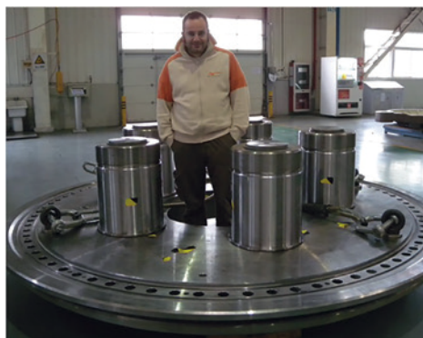
Figure 4—Upscaled carrier design, bearings and planet gears not yet mounted onto the Flexpins. Planets and bearings not yet assembled, for a 6 MW MGB.
